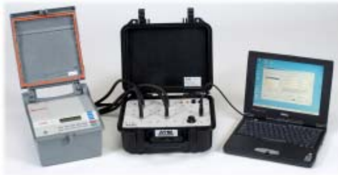
Figure 2 Setup of the ATRT 1150 with a Peek ADR-2000
