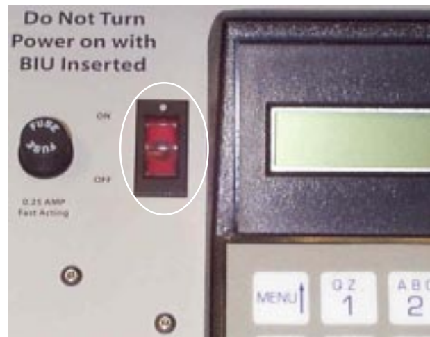
Figure 2: BIUT-800 tester power switch off
